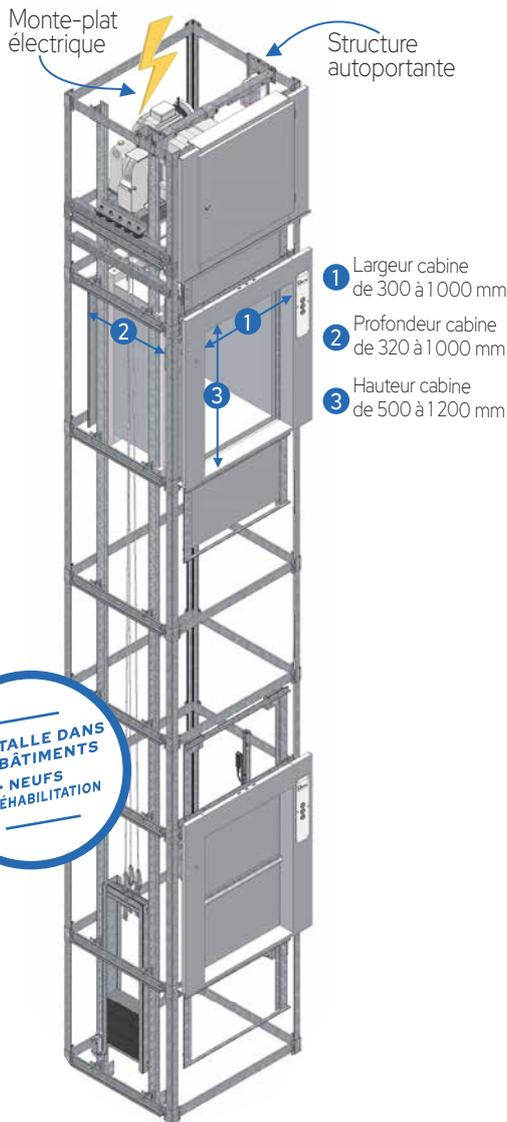
Conforme aux normes EN81-3 / directive machine 2006/42/CE
